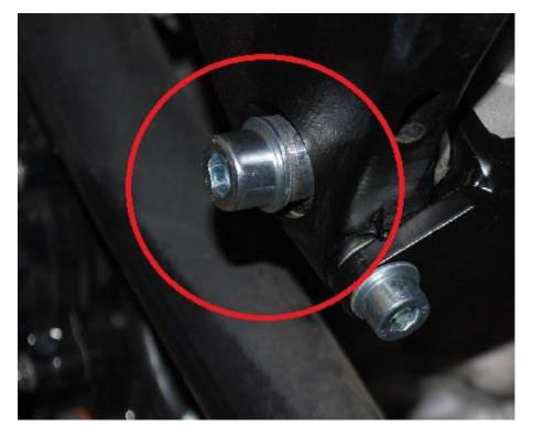
You will have to drill the hole in the cowl during installation. It is therefore necessary intervention in the original cowl!
