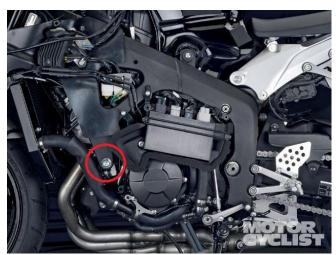
You will have to drill the hole in the fairing during installation. It is therefore necessary intervention in the original cowl!
