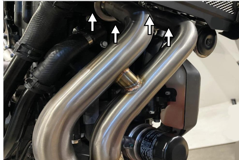
2. Tighten Lambda sensor into the manifold.
