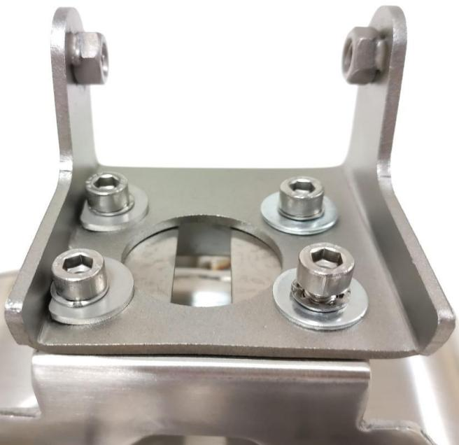
5. Tighten 4 x M6x16 before connecting with manifold.
