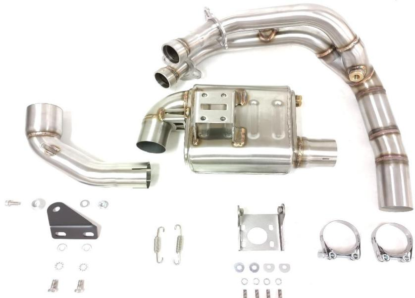
1. Assemble main manifold and just hand tighten 4 x stock cylinder nuts.
