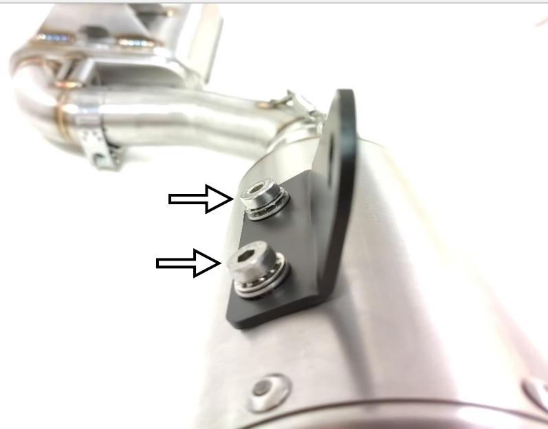
13. Fasten and hand tighten SOP7262 muffler's bracket to the footrest fender using 1 x M8x16 screw, 1 x EMBM8 screw cover, 1 x ARANM8 washer & M8 nut, as shown below.
