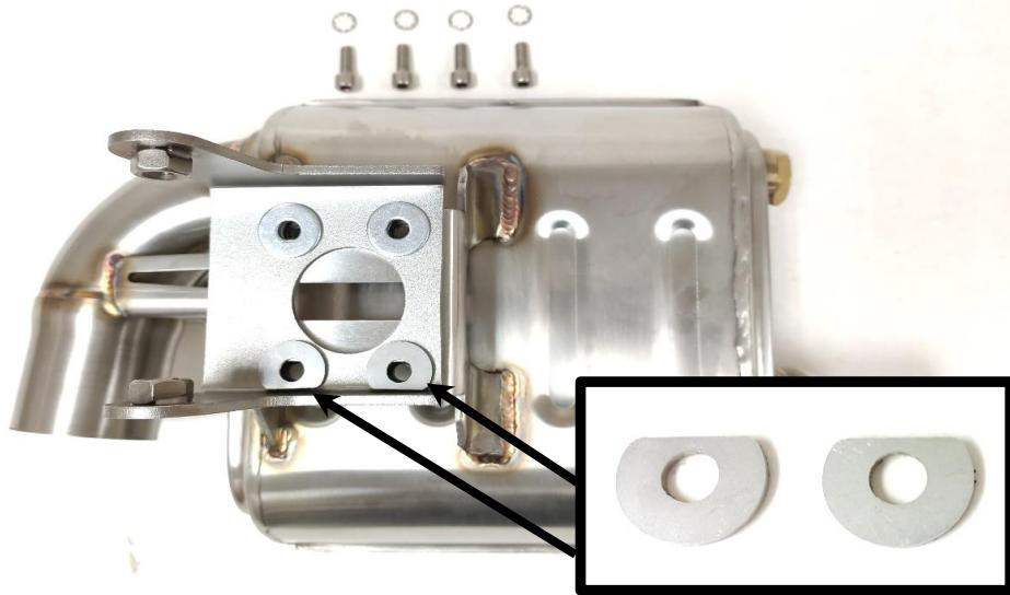
4. Under engine catalyst box bracket's mounting detail.
