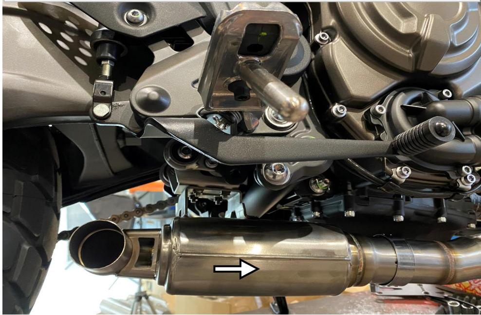
8. Mount cat. box to the frame's bracket, hand tighten, using 2 x stock bolts.
