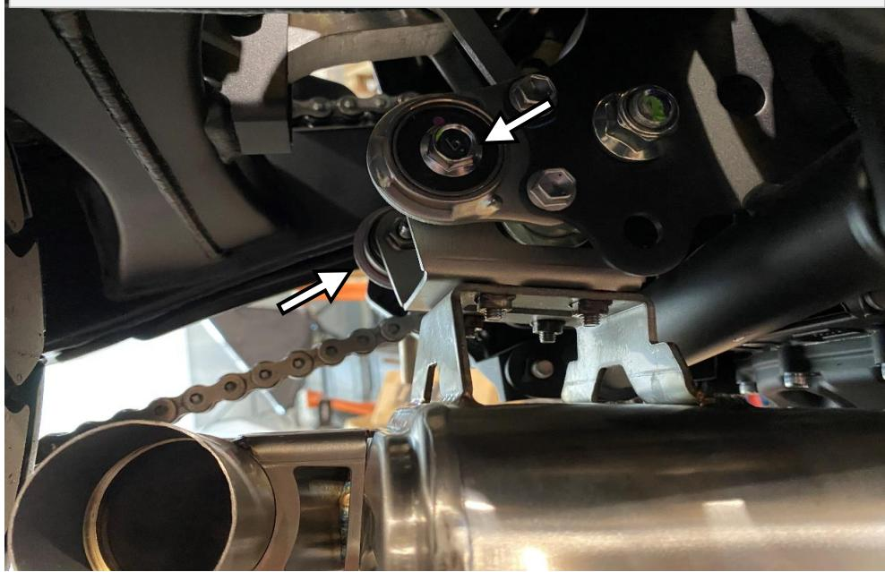
9. Place C5155 metallic flange onto the KIT7653T link pipe to connect with cat. box.
