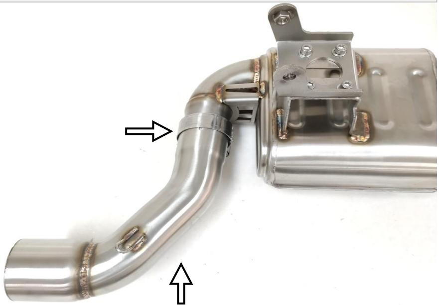
10. Catalyst box and link pipe mounting details.
