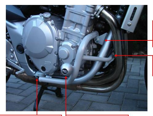
steel bolt M10x240mm + two pads M10 + two nuts M10
